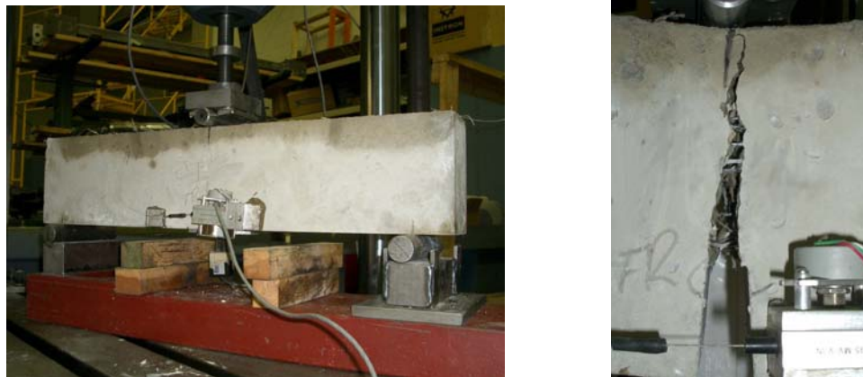
Figure 8a and 8b: Experimental set up of three point bending test and synthetic fibers bridging the crack
