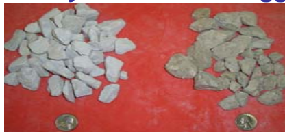
This figure shows virgin aggregate (left) and RCA (right)
